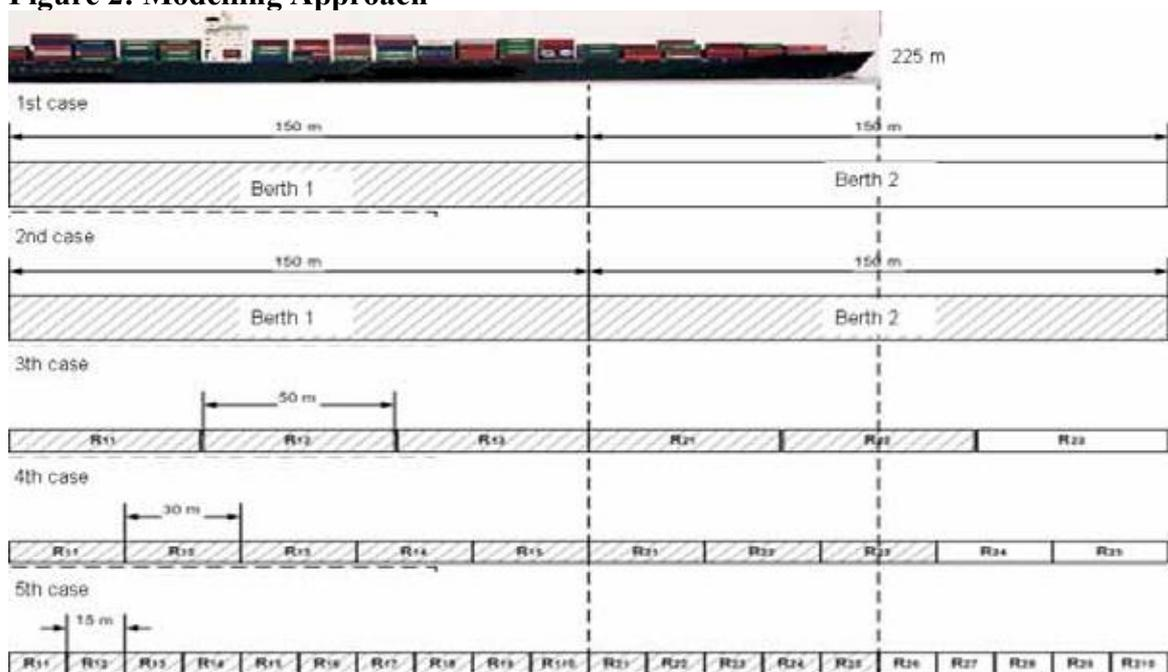
Figure 2 provides five alternatives of approach at quays from the view point of simulation modeling. A ship with a length of 225m (ship type no4) is assumed to approach the first two quays (Figure 1) of Port of Alsancak Container Terminal.
